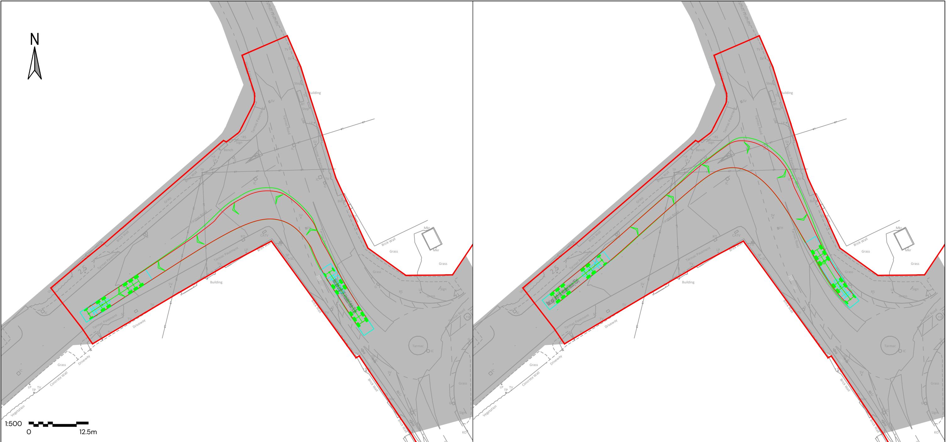
Swept Path Analysis of a 16.5m Articulated Vehicle Navigating Location V
