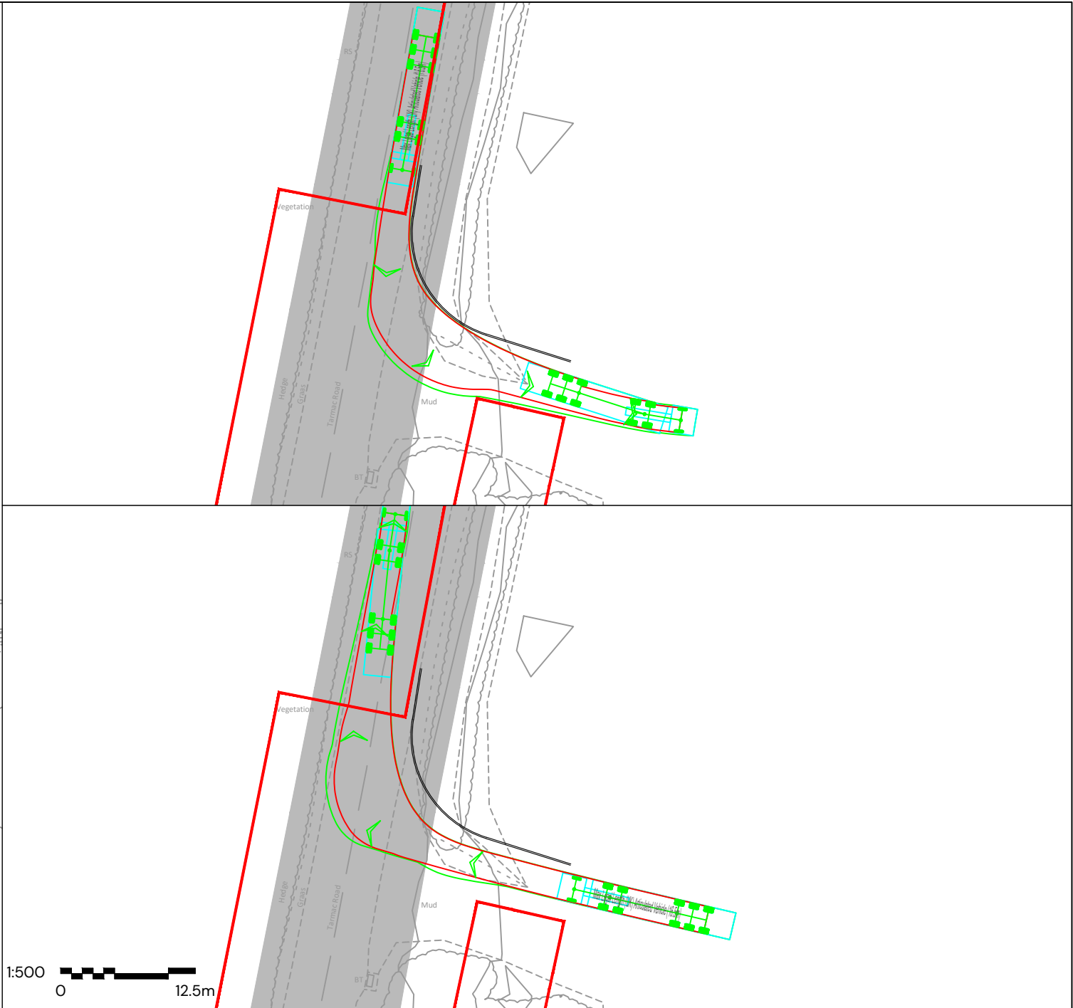
Swept Path Analysis of a 13.7m Tractor and Trailer Entering and Egressing Location Q Scale @ 1:500
